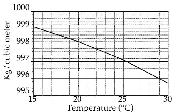
Figure 1. Density of water vs. temperature.
